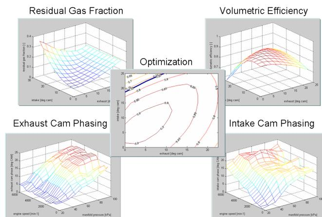
The entire data acquisition and optimization process takes less than half a day. The procured look-up tables reflect optimized calibration values which are close to the targeted production standard. They are validated and fine-tuned in a final empirical calibration step using an engine test cell.
